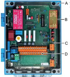
A AMI TransmitterB Slot for interfaces
