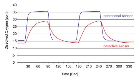
Unusual sensor performance is recognized immediately and gives also a maintenance indication to the operator/user. The faraday verification is therefore an excellent QA/QC tool.
