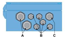
**A** PG 11 cable gland: cable  $\emptyset_{outer}$  5–10 mm **B** PG 7 cable gland: cable  $\emptyset_{outer}$  3–6.5 mm **C** PG 9 cable gland: cable  $\emptyset_{outer}$  4–8 mm
