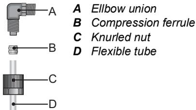
Connect the tube to the sereto elbow union and Insert it into an atmospheric drain of sufficient capacity.
