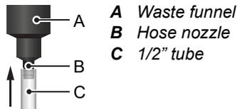
Connect the 1/2" tube [C] to the hose nozzle [B] and place it into the atmospheric drain.
