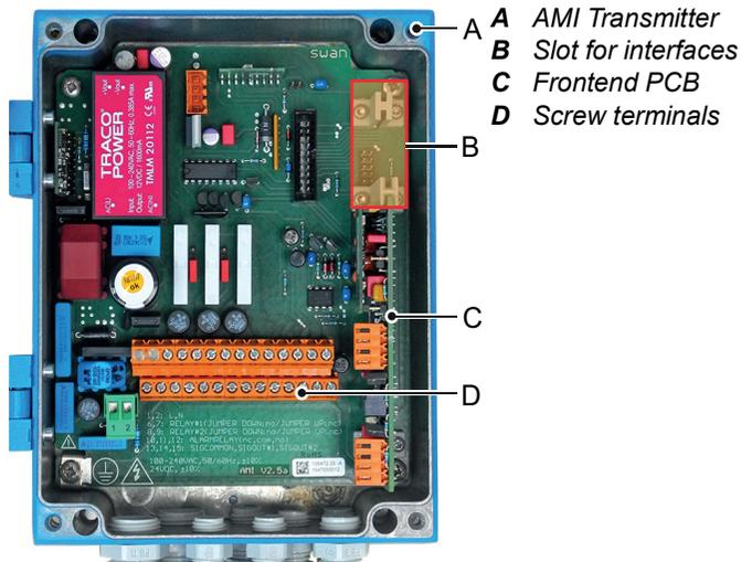
The slot for interfaces can be used to expand the functionality of the AMI instrument with either:
