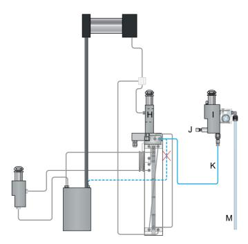
H Flow cell 1 of CACE Degasser K 170 cm FEP tube
