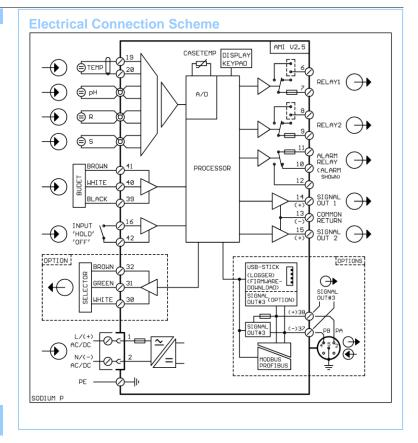
Overvoltage protection of in- and outputs. Galvanic separation of measuring inputs and signal outputs.
