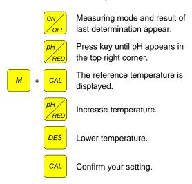
You can change the reference temperature any time. Only a new calibration will result in the temperature being reset to 25° C.
