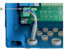
A 0.8 AT/250V Instrument power supply
