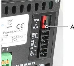
*A Switch for terminating resistor*
