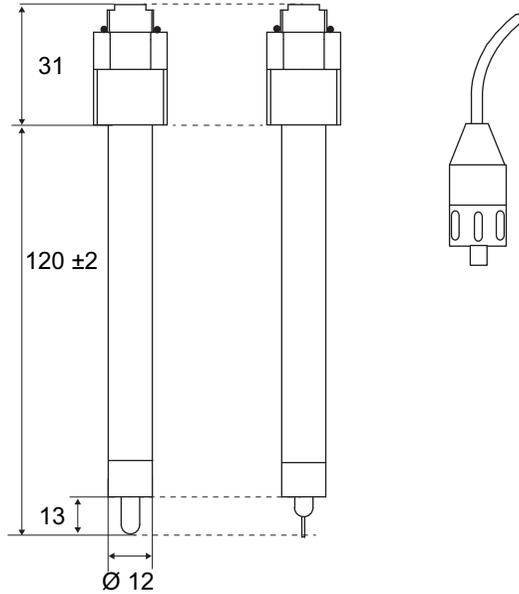
**pH Sensor      Redox Sensor      Sensor cable with plug**
