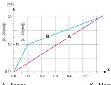
A linear X Measured value B bilinear
