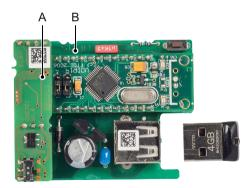
Signal output 0/4-20 mA PCB
